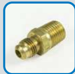
C10770 MALE PIPE CONNECTOR Material: Brass Fitting End A: 1/4" (-4) SAE 45° Male Fitting End B: 1/4" (-4) NPT Male
