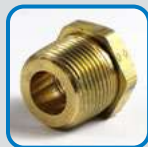
HP1238 BUSHING Material: Brass Fitting End A: 3/4" (-12) NPT Male Fitting End B: 3/8" (-6) NPT Female
