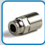
HP1210 FEMALE PIPE CONNECTOR Material: Nickel Plated Brass Fitting End A: 1/4" OD Tube Fitting End B: 1/8" (-2) NPT Female NON-DOT
