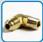
C10680 MALE PIPE 90° ELBOW Material: Brass Fitting End A: 1/4" (-4) SAE 45° Male Fitting End B: 1/8" (-2) NPT Male
