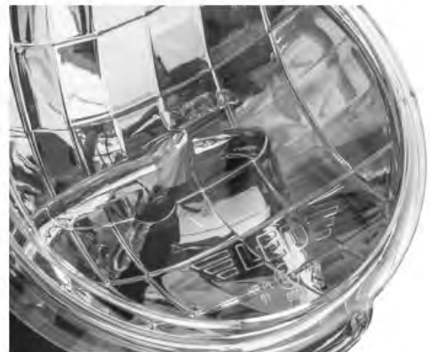
REFLECTOR FACING LEDS
