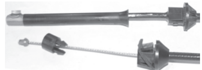
CA-8652 Description: Accelerator Overall Length: 28.5 Mounting Length: 22.25
