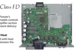
Large Capacitor and Plate-Type Heatsink
