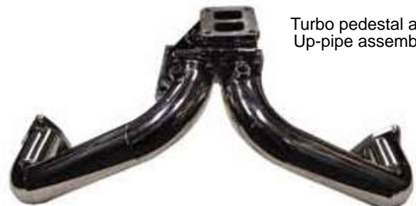
Duramax LBZ Marine Engine with Turbo pedestal and Up-pipes assembly and heat shields.
