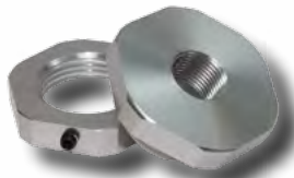
PN 4120473 - MODULAR FITTING ADAPTER, Billet Aluminum, Screw-In Type w/ Tapped Bore Hole, For 1.250" Hole, Includes 3/8" NPT to 3/8" Barb, Silver Anodized w/ O-Ring Seals
