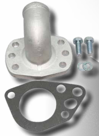
PN 5244081 - MOPAR, Cast Aluminum 90°, all V6/Slant 6/V8, As-Cast
