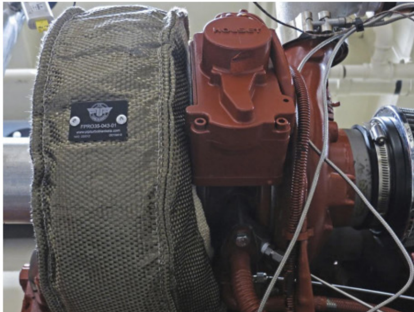
Figure 2-2 Unchanged tight fit of the PTP turbo blanket with temperature probes underneath it.
