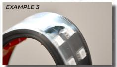
While this part contains a tough outer shell, there is no resin material encasing the circuitry or diodes. Once this seal is compromised the sensitive components of the light bar will be exposed to moisture and dust guaranteeing failure.
