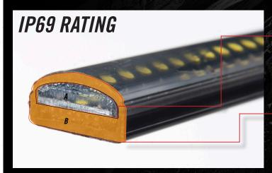
Patented 2-part resin conceals, protects, and insulates the circuitry. The custom resin is injected into the patented extruded housing in a vacuum, removing all air and
