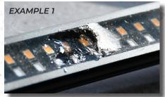
The material protecting the delicate circuitry and diodes from outside elements is only effective when intact. The soft resin material is easily scraped and removed exposing the diodes to moisture and dust. The exterior housing does little to prevent damage to the lens area on this particular light bar.
