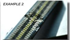
Again the product used to protect the circuitry is exposed to the elements and easily damaged. Once the fragile board and diodes are exposed to moisture, it is only a matter of time before component failure.
