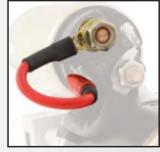
Wire jumps power from the solenoid to the starter when starter is engaged. Choose from wires with spade or ring style terminal ends.
