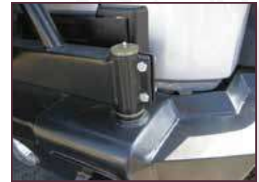
Adjustable, easy swivel hinge with grease fitting.
