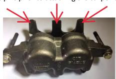
Apply a thin coat of brake lube to the outboard caliper casting where it contacts the brake pad.
