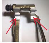
A thin coat of lube should be applied to the surface of the abutment clips where the brake pads ride on the clips.
