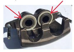
A thin coat of lube should be applied to the face of the caliper pistons where they contact the inboard brake pad.
