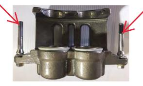
Apply a generous amount of lube on the caliper slide pins prior to attaching the caliper bracket.
