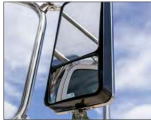
Motorized glass angles vertically and horizontally with 4-way actuator
