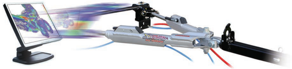
An engineering drawing shows the ‘hidden’ front arms (see page 9) and a portion of the receiver brace, which is attached behind the fascia. Every ROADMASTER baseplate is a custom design. This one fits the 2013-2019 Ford Flex.
