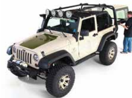
Designed to allow removal of hard top without moving the roof rack.
