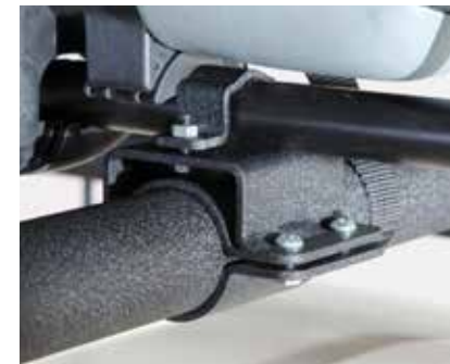
Use the optional Roof Rack Adapters to mount cross bars.
