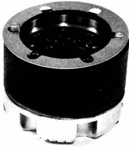
Figure 9 1001-19 Assemble outer gasket. Assemble lockout hub housing by aligning the splines of the housing with those of the outer clutch gear as shown. Assemble inner gasket on hub housing.
