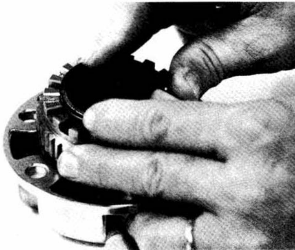
Figure 6 1001-16 Assemble pressure spring and outer clutch gear. Compress the pressure spring by forcing down on clutch gear and assemble snap ring. Make sure snap ring is secure in the groove of the cam. Turn actuator knob to free position.
