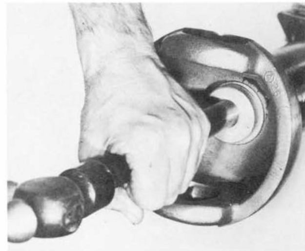
Figure 3-12 Assemble new bronze bushing into ball yoke.
