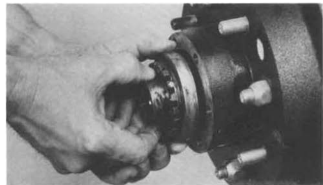
(Figure 10) Assemble bushing and inner clutch gear onto axle shaft, making sure the splines of the inner clutch gear are aligned with the splines of the axle shaft, as shown.
