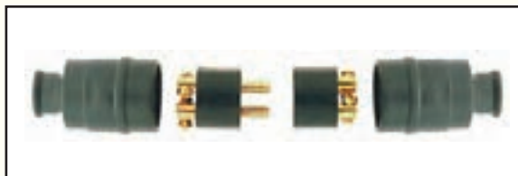
TC42 (Set) 4-Pole Trailer Connector • Hard rubber body, soft rubber end caps • All brass, metal components, polarized • Accepts up to 12 ga. wire
