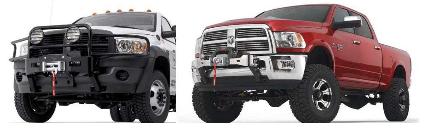
Ram HD equipped with WARN Gen II Trans4mer Mounting Kit, Grille Guard Tube (tall version), Headlamp Guards, and Light Bar
