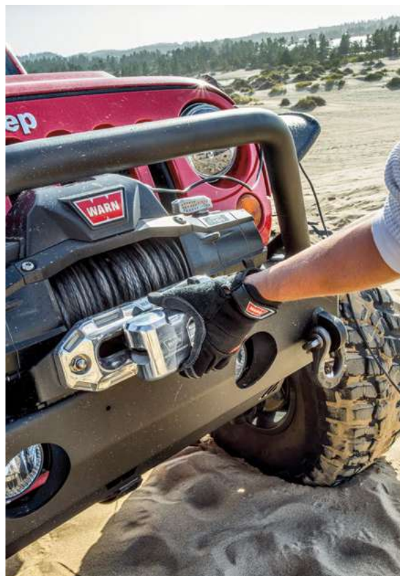
Sidewinder is designed to nest securely against fairlead when not in use for a clean look.
