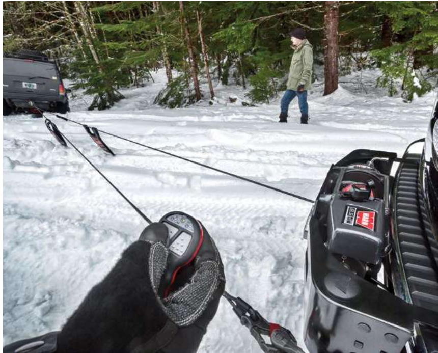
Receiver plugs in where you'd normally attach your corded remote
