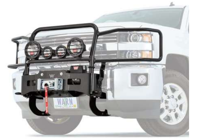
Chevy Silverado HD equipped with the large frame winch carrier, grille guard tube, headlamp guards, and light bar
