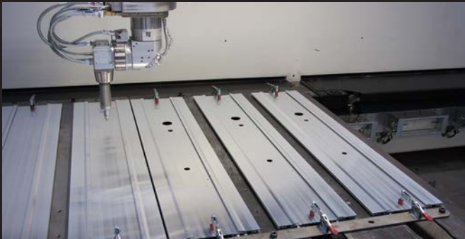
Sheet metal fabrication utilizes lasers to create brackets and a wide variety of metal components used in almost every Whelen product. A five axis laser is used to cut complex metal parts that do not come in a flat sheet.
