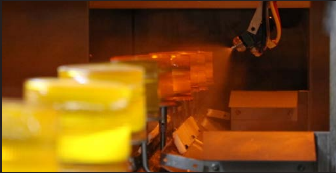
Hard coating technology utilizes an automated line where UV, abrasion, and chemical resistant coating is applied to all plastic lensing.
