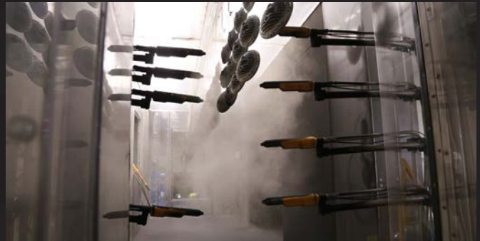
Powder coating technology uses an automated line which washes, dries, applies powder, and oven bakes.
