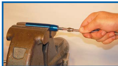
STEP 2 Flare braid using a twisting motion.
