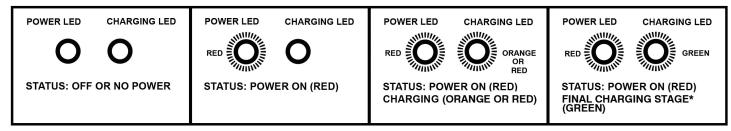
\*The LED Status Indicator will illuminate green indicating the final charging stage and a 1 hour minimum in this stage is required, however 24 hours is recommended for 100% charge.
